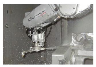
LR Mate 200iB/5WP with ingress protection is used for high-pressure washing of parts or for packing food.
