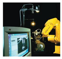
Precision jewelry polishing system with part shape recognition uses FANUC's V-500iA/2DV Vision System.
